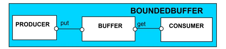
The behaviour of BOUNDEDBUFFER is independent of the actual data values, and so can be modelled in a data-independent manner.
