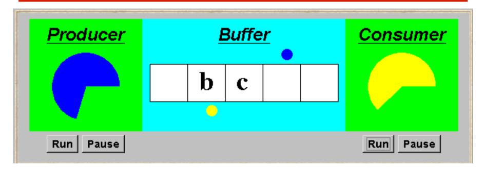
A bounded buffer consists of a fixed number of slots. Items are put into the buffer by a *producer* process and removed by a *consumer* process. It can be used to smooth out transfer rates between the *producer* and *consumer*.
