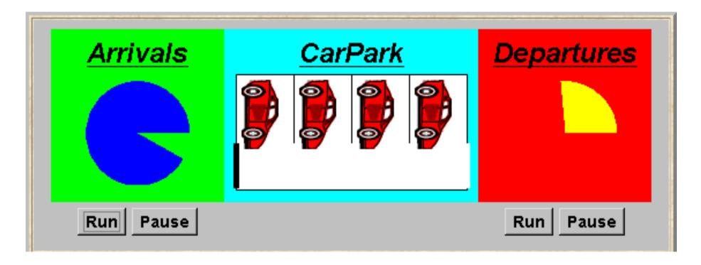
A controller is required for a carpark, which only permits cars to enter when the carpark is not full and permits cars to leave when there it is not empty. Car arrival and departure are simulated by separate threads.
