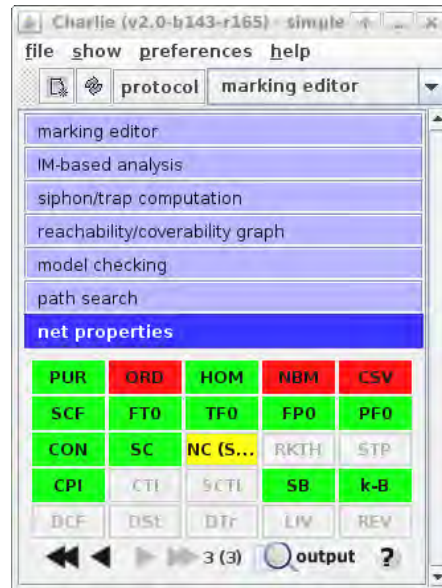
Fig. 1. A screenshot of Charlie’s GUI showing the standard features without any extension. Starting from the top one sees the menu bar, followed by some buttons for a quick access to often used functions and the dialog boxes for the different analyzers. At the bottom a special dialog appears, the “net properties”. This dialog shows all properties Charlie knows of. If the loaded Petri net fulfills a property then it is marked in green, if the Petri net does not fulfill a property then it is shown in red. Unknown properties, i.e., properties that have not been analyzed yet are shown in gray, while a yellow color indicates that more information than true or false are provided. Finally, there are control buttons to switch through the different results and to show the “output” and “help” windows.
