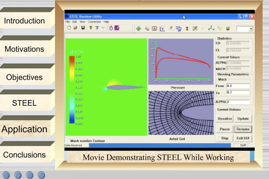
Numerical flow Simulation and Visualization past an Airfoil at Transonic Speeds
